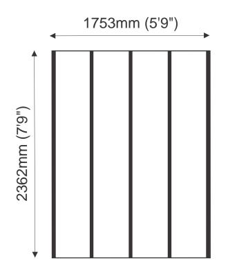
If using bearers we suggest 4 at 6ft (1.8m) We reserve the right to alter design without prior notice. If it is crucial that the floor joists run the same direction as shown above, this must be stated on the order.
